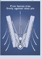
**DISC SEAL OVERLAP:** Contact between the seal and the disc is uniquely designed to eliminate indentation ridges found in designs
