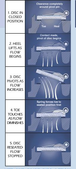
**LIFT AND PIVOT DISC ACTION:** This feature, designed to give longer valve life, is activated during the opening and closing cycles. It works by a combination of clearance between the pivot pin and disc bores, and the placement of the legs of the torsion spring. With this design the disc will always lift first at the pivot on opening, and not return until the disc is closed, preventing wear between disc and seat surfaces.
